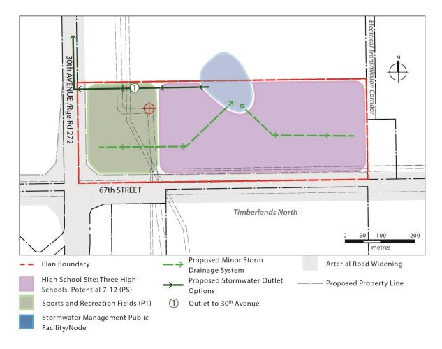
North East High Schools & Playfields Site Area Structure Plan Stormwater Servicing - Minor Storm Drainage System and Outlet Options
