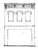
**Cornice** - traditional building cornice, made of stone, brick, wood, metal, or other materials; serves to visually cap the facade.
