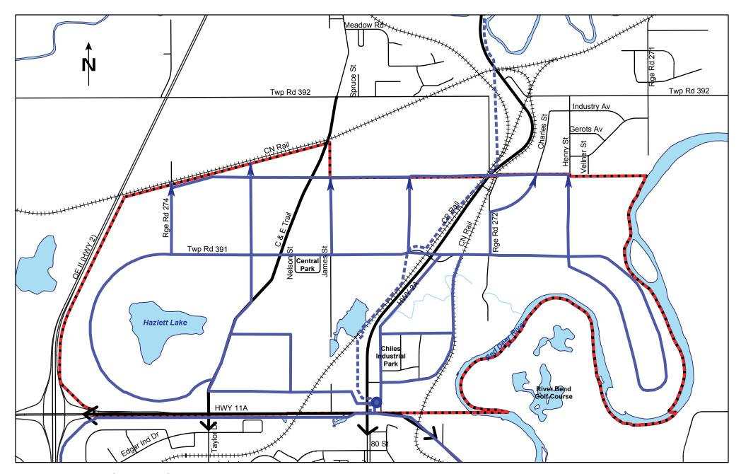
Figure 10: Water Servicing Concept North of 11A MASP
