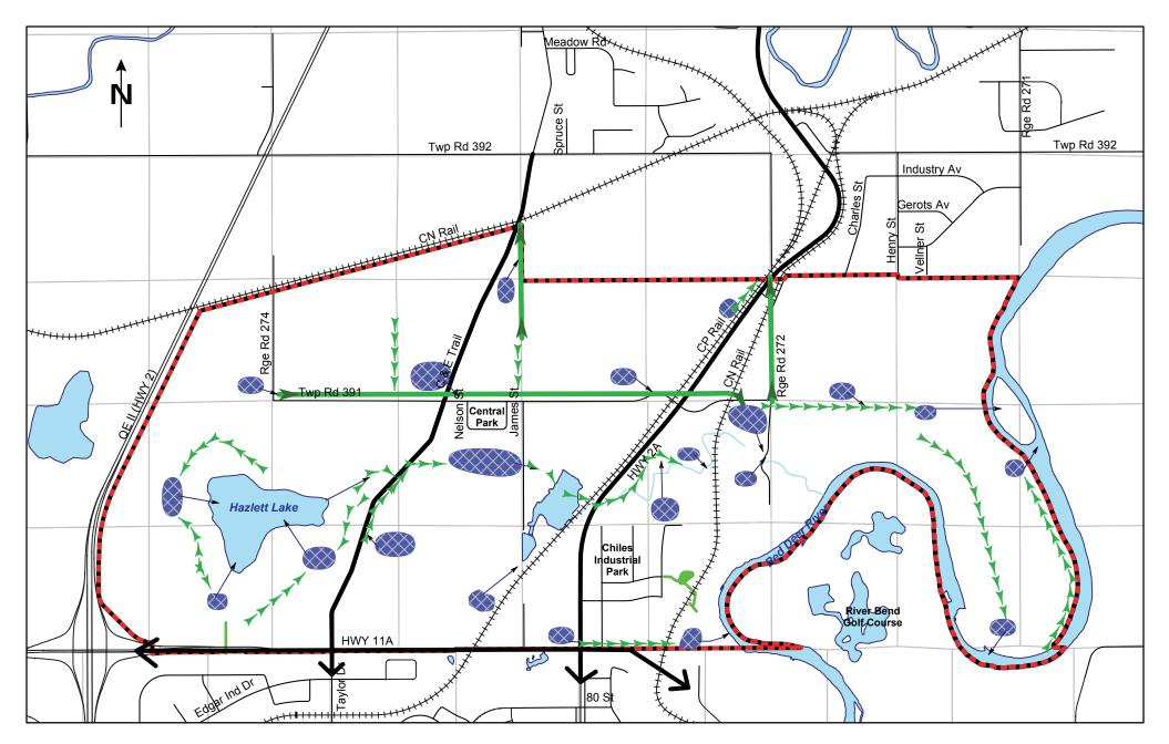
**Figure 8: Storm Servicing Concept** North of 11A MASP
