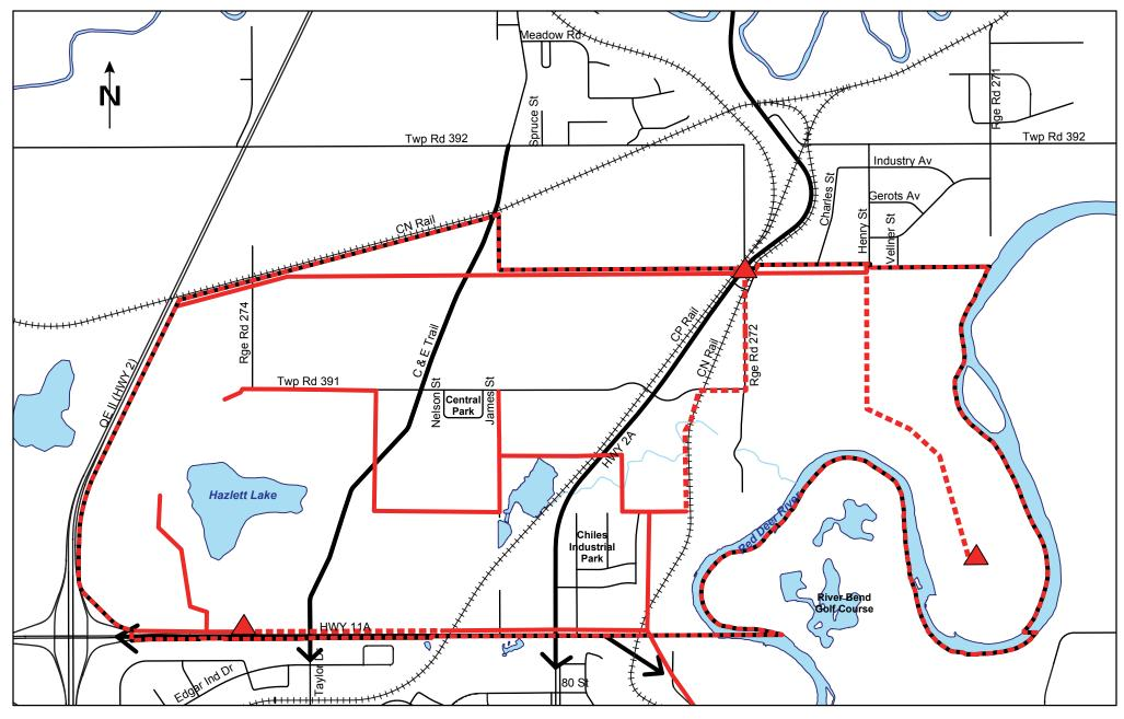
Figure 9: Sanitary Servicing Concept North of 11A MASP
