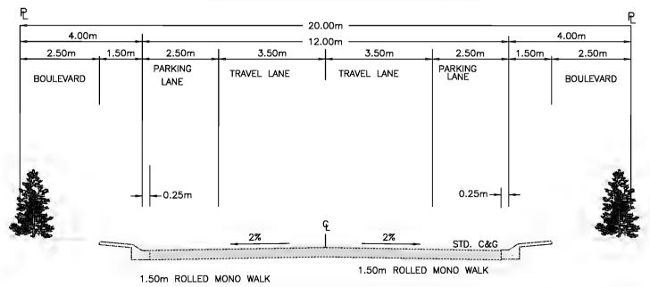
FIGURE 13 DIVIDED AND UNDIVIDED RESIDENTIAL COLLECTOR ROADWAY DETAIL
