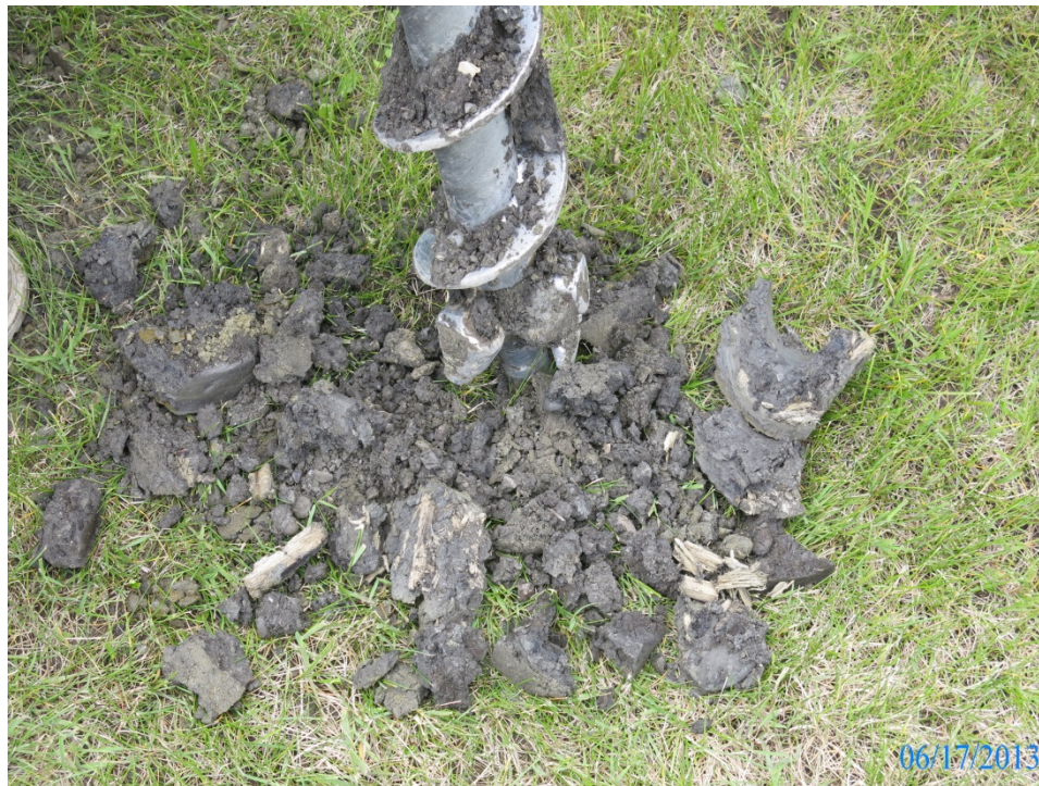
Photograph No. 4: View of drill cuttings at TH-01. Note wood fragments only mixed with cuttings from 5 m to 6.1 m.
