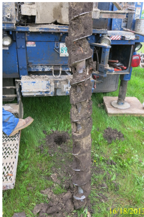
Photograph No. 12: Small amount of wood fragments in the drill cuttings from a depth of 1.5 m to 3 m at TH-10. No other waste material encountered.
