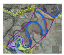
Illustration of a floodplain based on SRD delineation of a meander belt.
