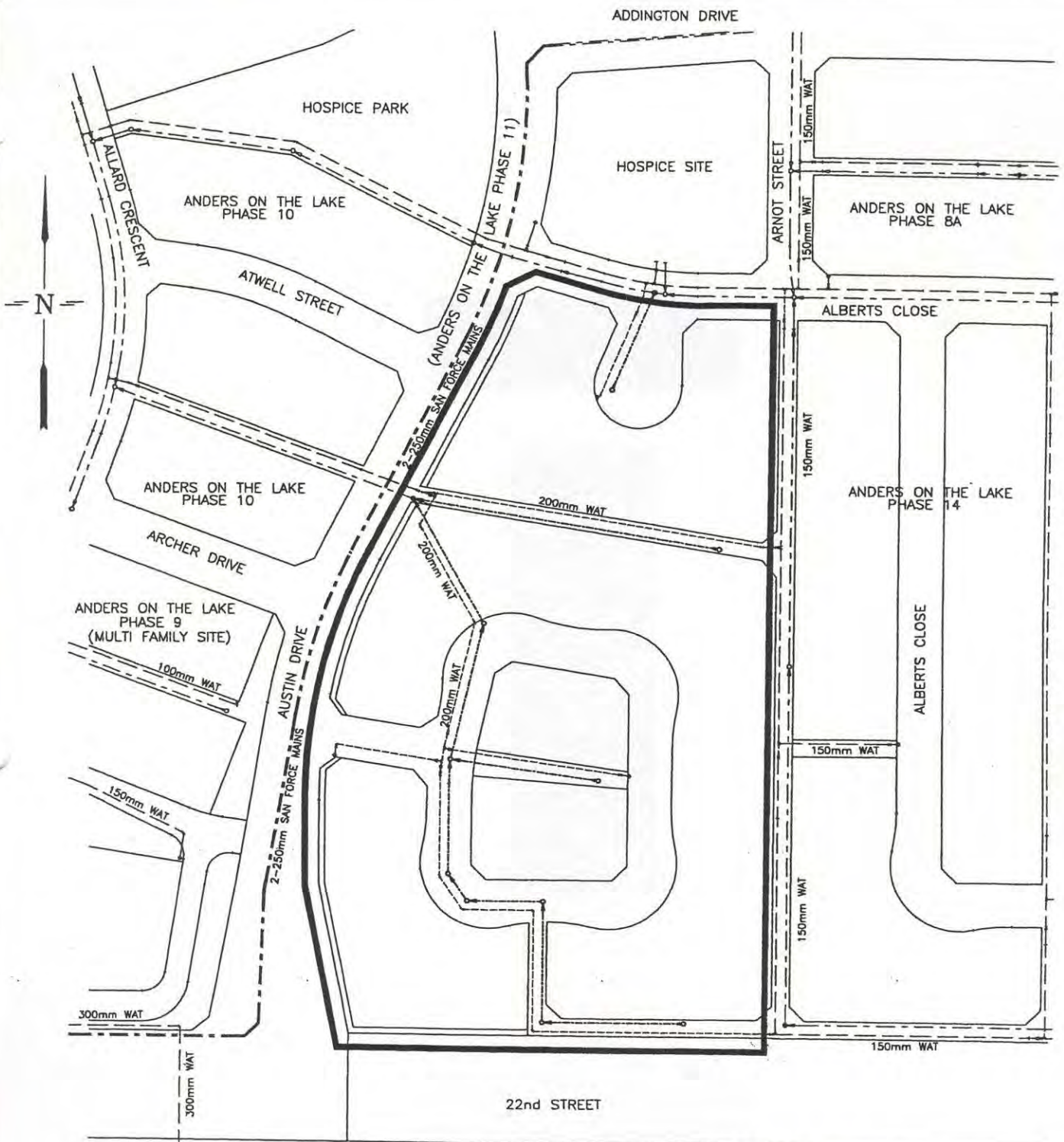
FIGURE 4 ANDERS ON THE LAKE DMC CONSTRUCTION SITE SITE SERVICING - SANITARY SEWERS & WATER MAINS
