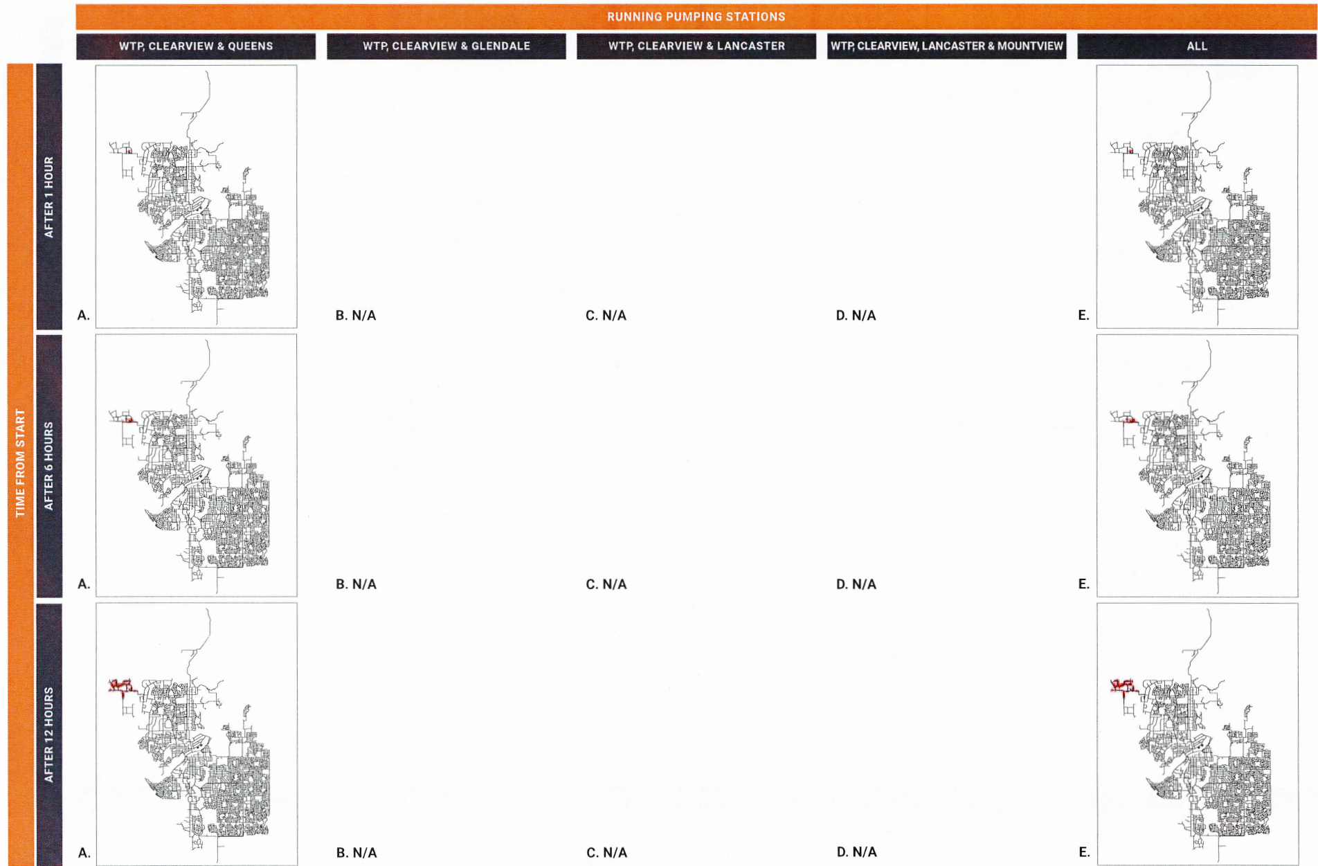
Figure C.3: Trace Analysis Results for the Queens Pump Station as the Trace Source under Average Day Demand Scenario
