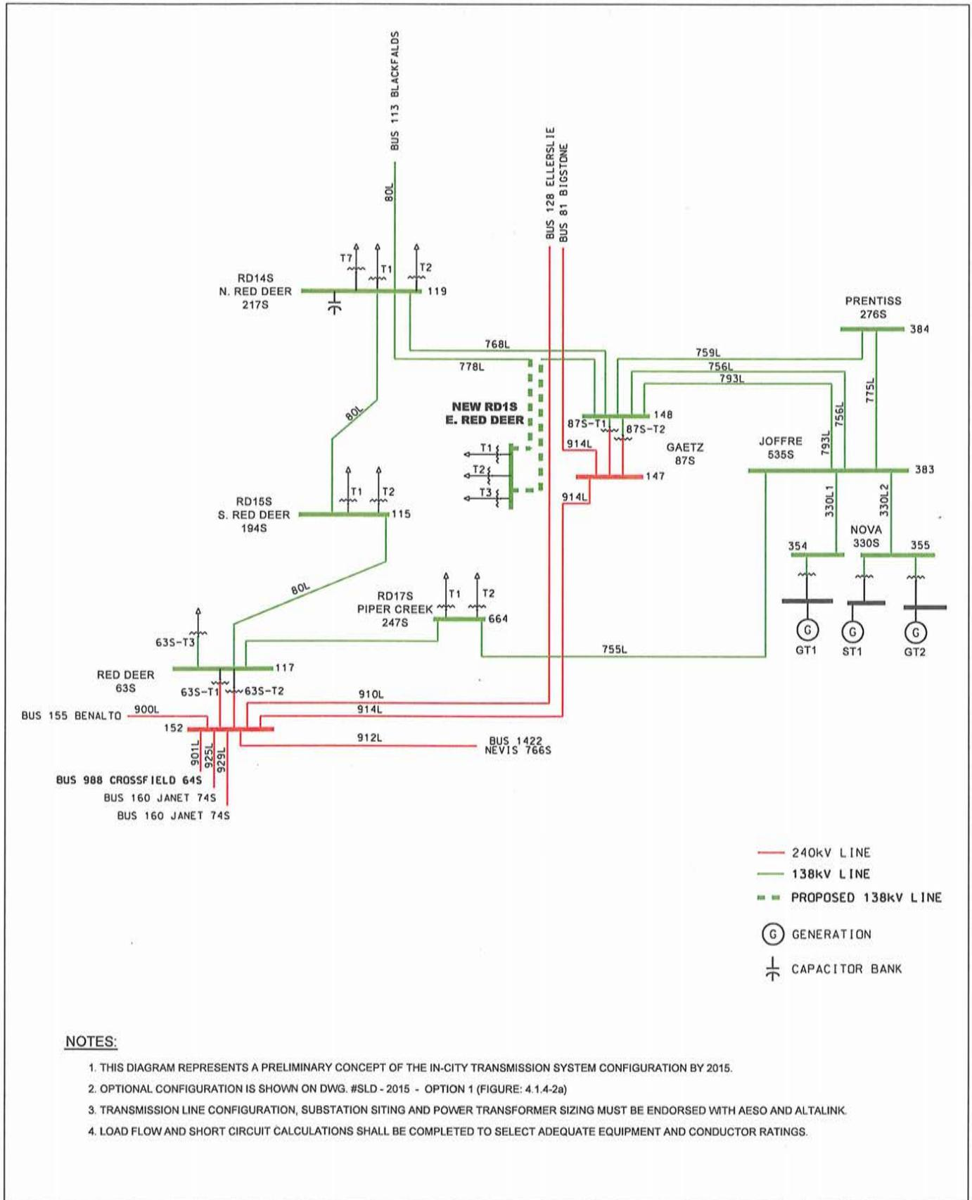
Figure: 4.1.4-4 In-City Transmission System Concept 2025 - Option 1
