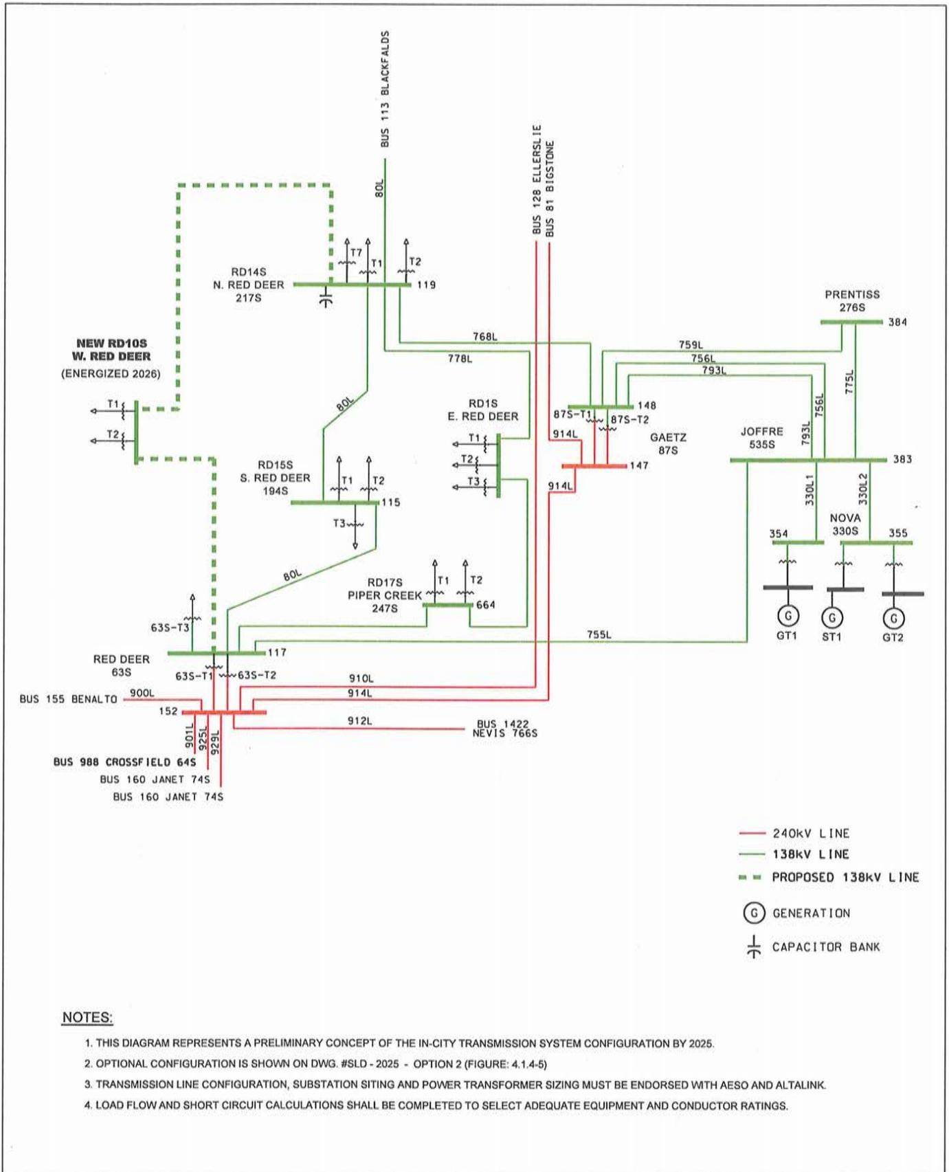
Figure: 4.1.4-5 In-City Transmission System Concept 2025 - Option 2
