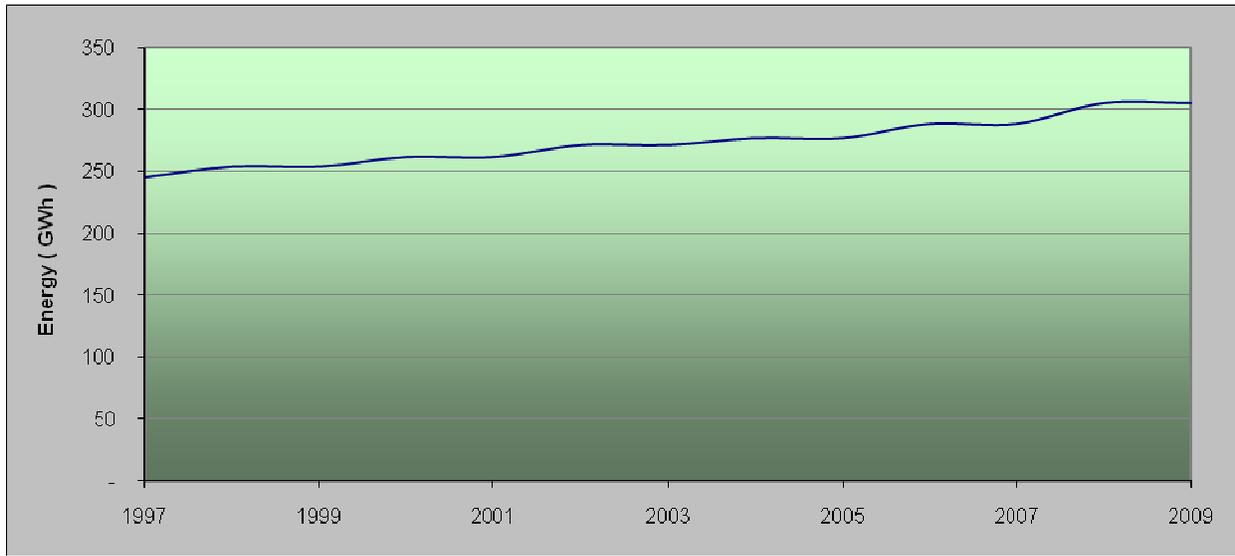
Figure 3.2-2 shows the hourly average electrical demand from 1997 to 2009 per customer per month for the commercial and large commercial sector. While the historical commercial electrical energy consumption shows a steady increase Figure 3.2-2 shows that the increase in electrical demand is not attributable to increase in consumption per customer.
