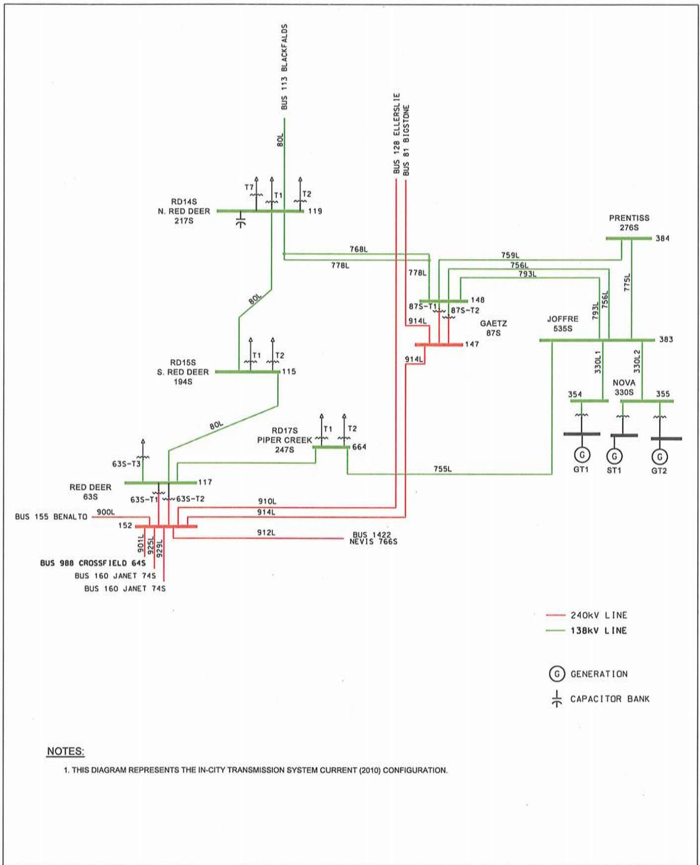
Figure: 3.2-1 Existing Distribution System Topology
