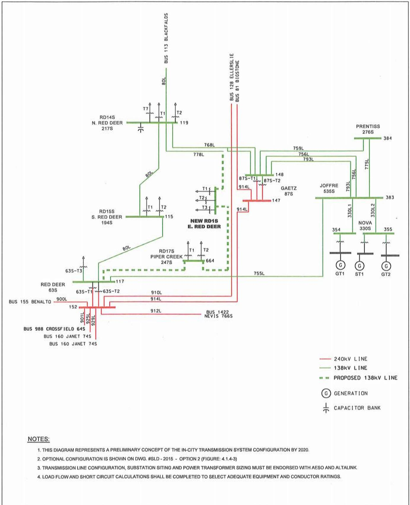
Figure: 4.1.4-3 In-City Transmission System Concept 2015 - Option 2
